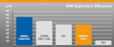
At 74 LPW, this lamp's efficacy is over 10% higher than the Tier 1 LED A19 40W replacement average and exceeds the new ENERGY STAR requirements by upwards of 35%. This energysaving performance makes this lamp a smart retrofit choice for incandescent and CFL bulbs.
