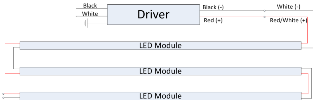
Figure 2: Daisy Chain Wiring
