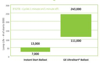
GE lamp life studies have shown that lamp life is up to 20 times longer in rapid cycle testing. Lamp life tests have demonstrated 111,000 to 243,000 starts on F32T8 lamps to rated lamp life with GE UltraStart® ballasts as opposed to only 7,000 to 13,000 starts with standard instant start ballasts. GE lamp warranty may be void if lamp starts exceed 3,000 starts during the warranty time period with instant start ballasts.
