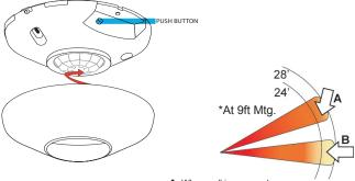
A: When walking across beam, detection will occur at approximately 28 feet. (8.53 m)
