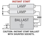
2. Re-wire fixture as shown below (maximum of 4 LED tubes per fixture).
