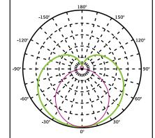
Maximum Candela = 1248.55 Located at Horizontal Angle = 0, Vertical Angle 0
